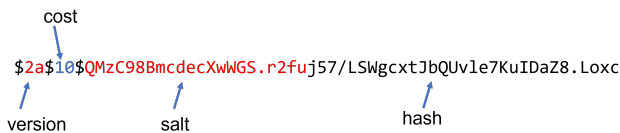
Fig. 4. The password hash format from Bcrypt algorithm.
